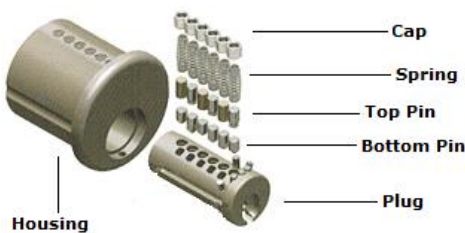
Figure 2: Cylinder pin tumbler
